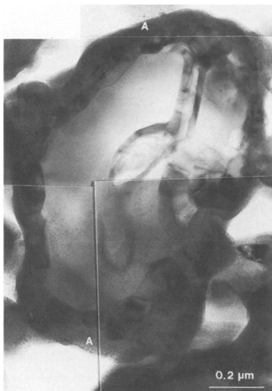
Figure 8 A silicon powder particle at an early stage of nitridation at 1350°C. Note the tunnels extending from the particle surface into its interior. The fine-grained surface layer and tunnel walls are probably newly formed \text{Si}_3\text{N}_4 grains. A thin amorphous layer (A) is coating the fine-grained structure.
